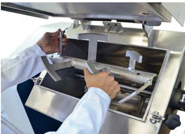
Detail of the detachable mixing shaft with blades
